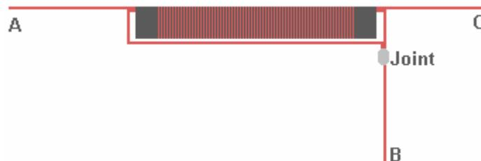
The coil needs to be checked carefully before use. Ideally, the joint is soldered and if the enamelled copper wire used is the "solderable" type (which is the most common type) then the soldering iron heat will burn the enamel away after a few seconds, making a good joint on what used to be fully enamelled
