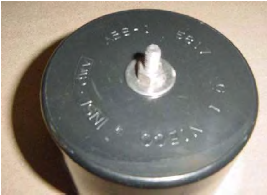
This is the Positive battery connection.
