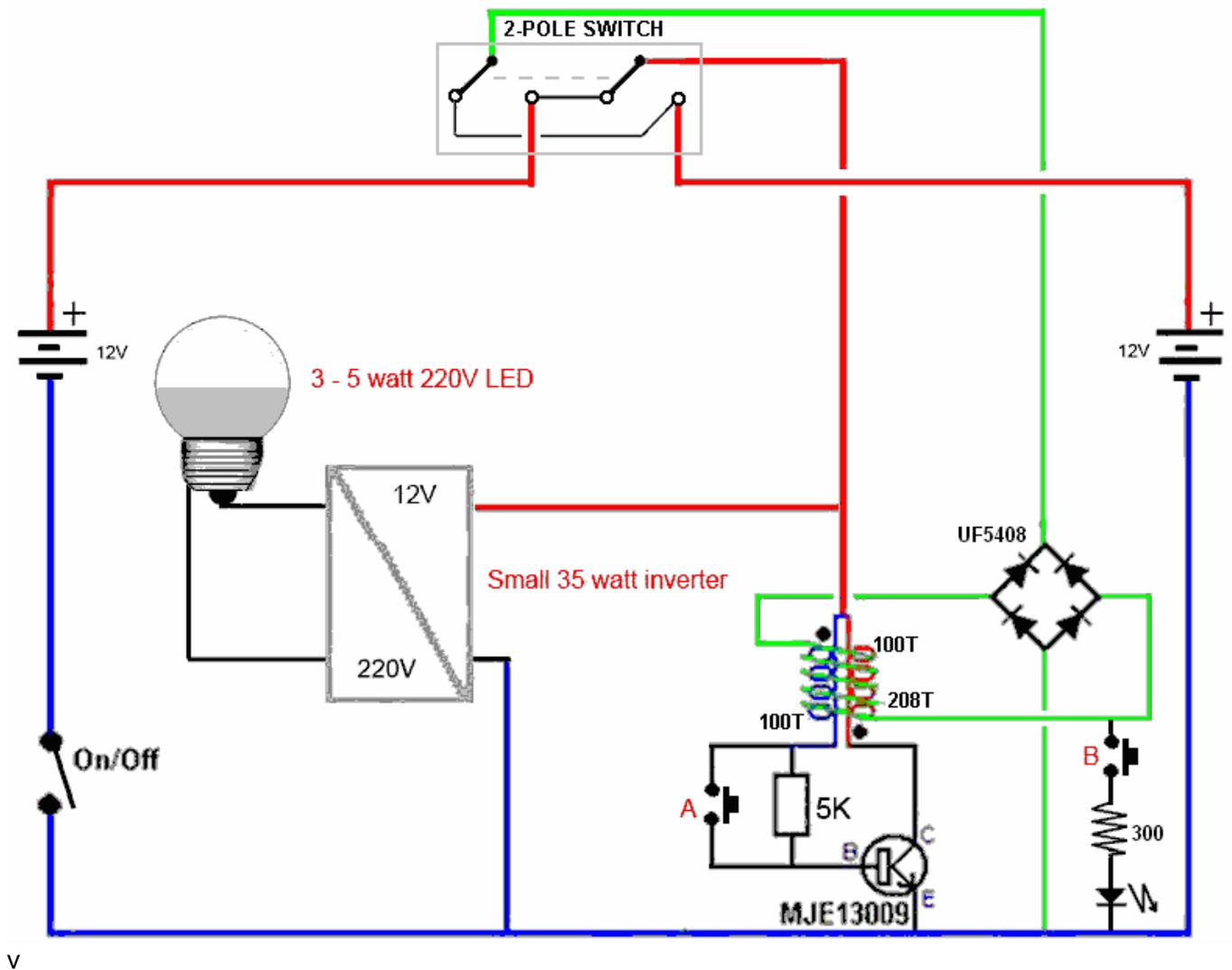
Pressing button switch “B” will light the indicator LED if the Joule Thief charging circuit is oscillating and if it isn’t running, then a brief tap on button “A” will get it running as that uses the blue winding directly to feed a large current to the transistor.
