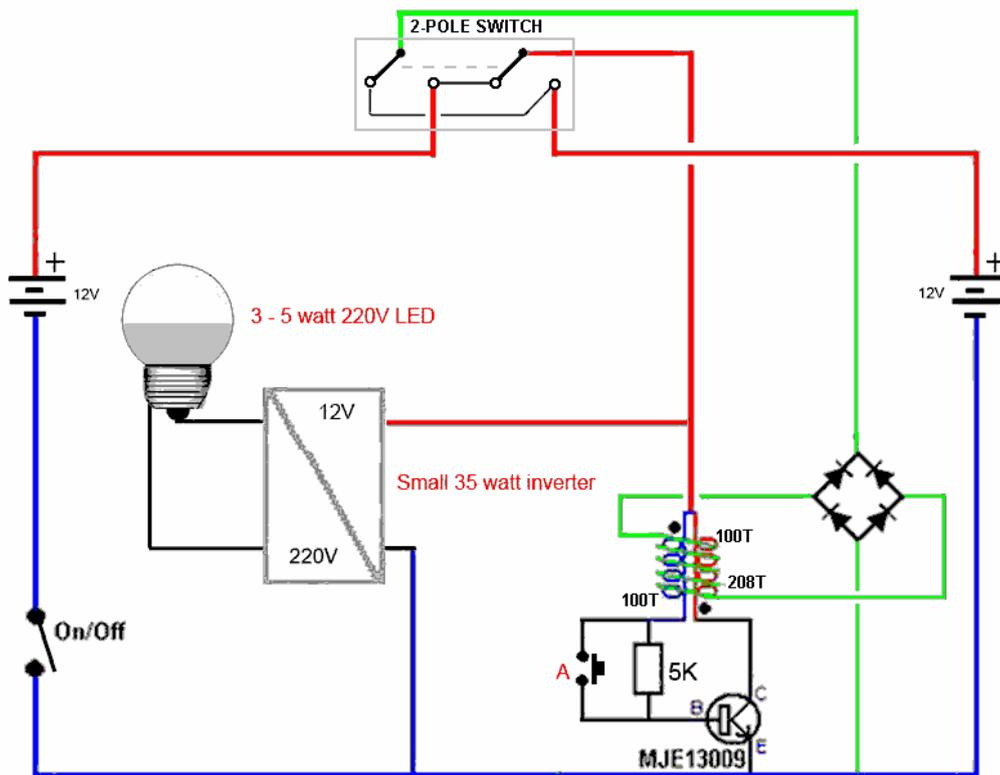
The charging circuit is an ordinary Joule Thief circuit with an extra FLEET-style winding shown in green. The voltage developed in that winding is rectified by the diode bridge and passed to battery which is being recharged. This light is always available and never needs external charging.
