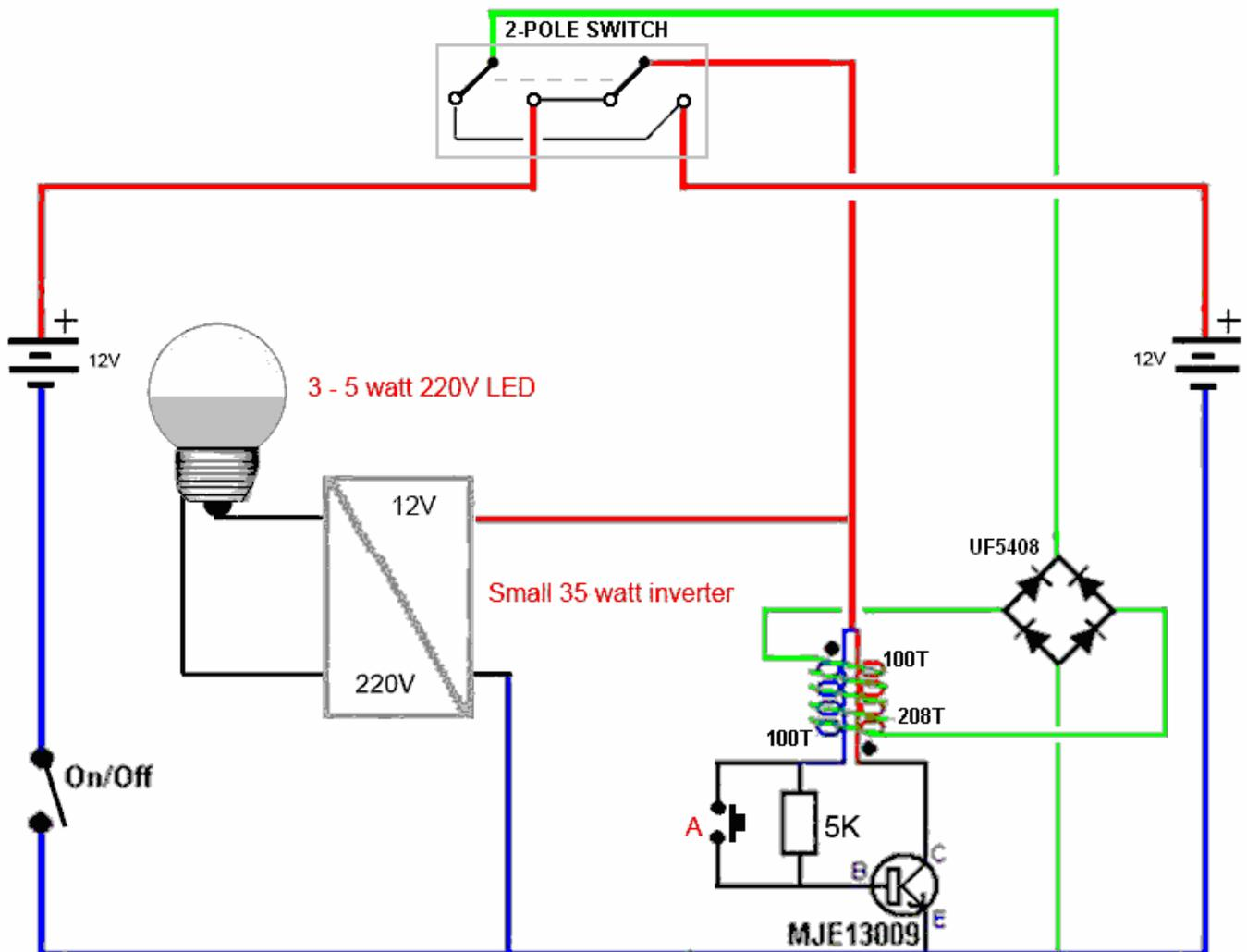
For the light, the developer has chosen to use a 220-volt bulb, rated at anything from 3 watts to 5 watts as that is easy to organise and gives really good lighting. Ignoring the coil circuitry, the circuit is extremely simple with a small inverter powered by either of the batteries.
